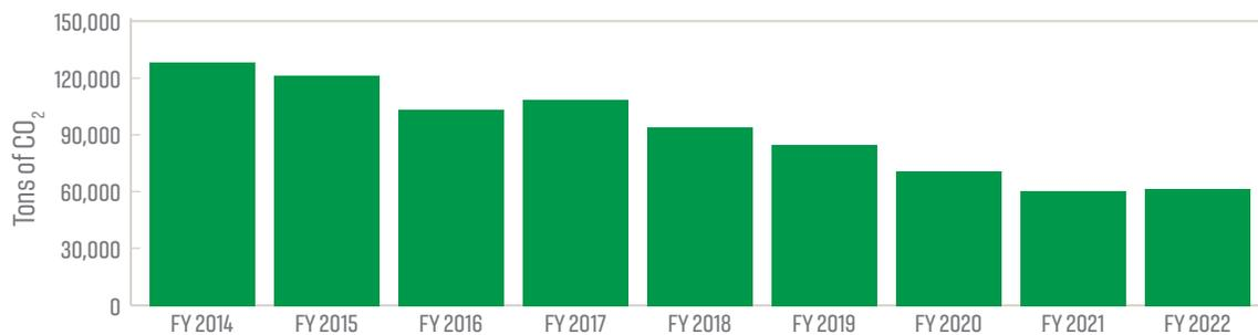
Figures 3 and 4 show power plant fuel consumption, usage, and GHG emissions between FY2014 and FY2022. Power plant GHG emissions have been reduced significantly since the change in fuel source to natural gas nine years ago. Fuel consumption at the power plant increased slightly from FY2021, which can be attributed to the campus reopening after COVID-19 closures and the recent campus area increase.
